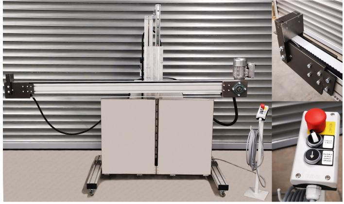
Lifting aid to lift raw profile bars onto roller conveyors or loading magazines by a single operator. Pneumatic lifting of the transport belt with an adjustable stops for the lifting heigth.
